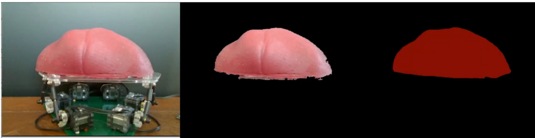
Figure 21: Segmentation in brightly-lit conditions
